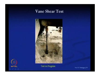
So, this is the vane shear test which is in progress; apply the torque in the soil.
