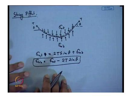
Next one is the string effect that is also very important. What membrane effect we can says, so that means the, if so there is a reinforcement pattern. So, here the T is developed here, here T is tension is developed and this angle is set theta, this angle is also theta. So, that means at the top of the reinforcement this force is acting, this is the normal force sigma n tau.
