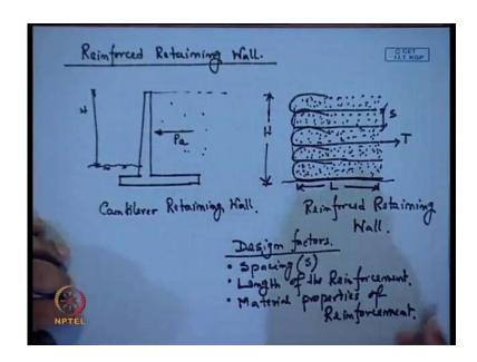
Now, this reinforced retaining wall, so we know this is our suppose, they are cantilever retaining wall. So this is a soil, this fill this side and this is the existing soil or foundation. Now here the soil is giving lateral pressure on the retaining wall, so this lateral pressure is taken by this cantilever retaining wall.
