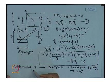
So, this is sheet pile; this is the top level; it is the dredge level; now this is the ground water table position. So, forces that is acting, this is the F anchor force; this force is p active; and this is p passive; this distance is D or depth. So, this is the a e o and b; and this point, this is the p active at e level; this distance is a, remaining one capital Y.
