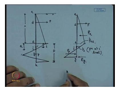
Now if I go for the pressure distribution diagram for this type of sheet pile, then we will get, suppose this is the sheet pile; this is dredge level. Now, the pressure distribution diagram, we are considering there is again, this is a; this is the anchor point d; this is e; and this is b; then one position is i which is point of contra fiction; then below that this is say g.
