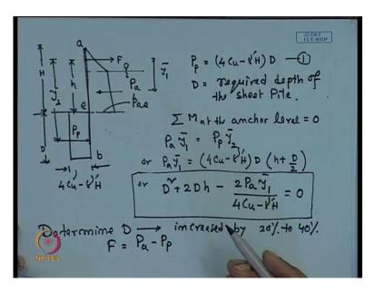
So, now, if I draw this same figure. So, we can draw this is the sheet pile; this is dredge level. So, this is water table position is here; this is anchor force F. So, here net pressure we have calculated this one is 4 c u minus gamma dash H. And this is the p a e that is e position; this is a; this is base b; and this is the rod level.
