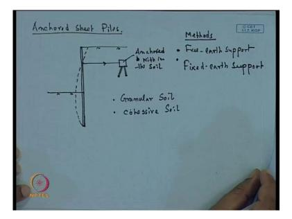
So, now first, if I go for this anchored sheet pile condition, similar to that this is the top ground surface; this one is the dredge level; and this is the cantilever sheet pile. Now here sometimes to reduce this required depth, one anchor is used here. So, this is this that means, this here apply tension is applied with the, this is the sheet pile, where this tension is applied through this anchor; then it is anchored in the ground.
