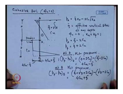
Now, here first expression of P A; that is equal to q bar into K a minus 2 Cu root K a. So, q into K a minus 2 Cu into root K a, K a is the coefficient of active earth pressure. Now where q bar is equal to effective vertical stress at any depth, and here phi u is 0, so your K a that is equal to K p, that will be equal to 1, as phi u equal to 0 for this expression, so K a equal to K p that will be 1.
