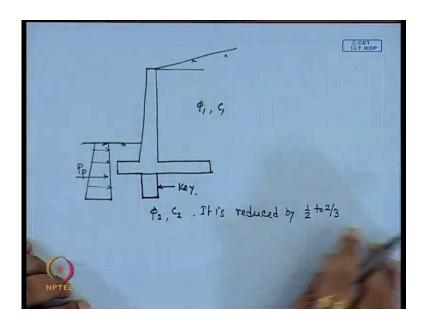
Suppose, this is our retaining wall structure. So, this is the retaining wall structure, ground surface, this is ground surface. Now, say this retaining wall is, unsafe against the sliding. Then one thing we can do that, we can provide one key here, in this form, just to increase this another portion, that we can exchange, it is called key. The idea of this key, this will give the additional resistance against the sliding. So, an another thing is that,
