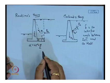
So, if I this is our foundation, this is the ground surface, this is backfill side. So, then we first, we if we use the first case, we will use the Rankine theory; and next one, if I use the coulomb's theory; so the same retaining wall if I consider for the coulomb's theory, for the different forces that you have to consider, that again if I join this point, so this is
