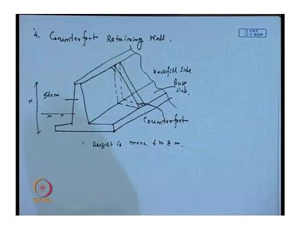
And the next one, another type of retaining wall is, that is counter fort retaining wall, where this is the retaining structure, and this is the longitudinal side, where with some interval this counter forts are used. So, these are called counter forts, this is. Now this type of reinforce, this type retaining wall, they providing. The use of this counter fort is to reduce the shear force, and the bending moment in the vertical steam of the slab. So,
