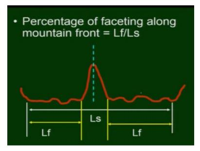
So about the triangular facets what you can do is you have one of the parameters which we were taking about the Ls that this traced length of the mountain front and you can have the divide here between the drainage and then you can have the left front and the right front and that can give you the percentage faceting, okay. So with the help of again Lf by Ls, you will be able to calculate the percentage of eroded fronts.
