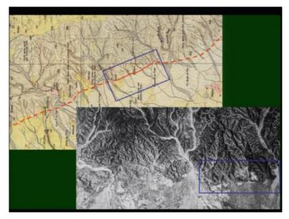
So as I told that one can extract the information from the topomaps and the high-resolution satellite data, so topographic maps usually have been prepared from the high-resolution aerial photographs or satellite photos and what we see in terms of the information on the topographic maps are the drainages and we have the contours which talks about the elevation in the area with respect to mean sea level. So if you look at these contours here, this is like 400 meters and then reduces further down.
