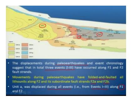
So based on the interpretation, using all the cross-cutting relationships along the fault and different fault trends and the ages we interpreted that at least 3 events have occurred along and we were able to identify at least three events along the Kaladhungi fault, that is an imbricated fault of HFT. So we say that the displacements during paleoearthquakes and the event chronology suggest that the total 3 events have occurred along F1 and F2 strands.
