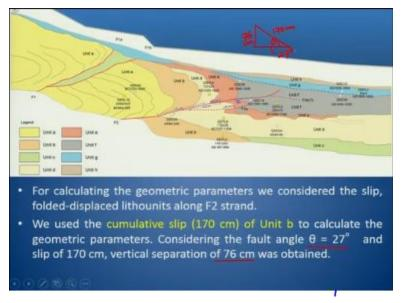
So for calculating the geometrical parameters, what we did was that we considered the slip one, folded and displaced the three units, along F2. So you wanted to go back into the deformation pattern and reconstruct how the deformation exactly took place. So, we use the cumulative slip of 170 centimeters of unit b to calculate the geometric parameters. So we used a very simple trigonometry here like for considering you have the fault angle here.
