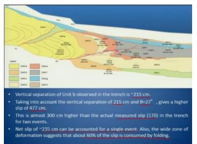
So the vertical separation of the unit b to be observed in the trench was 215 centimeter. Taking into account the vertical separation of 215 centimeter and the theta 27 degrees, gives a higher slip of almost 477 centimeter but actually the slip, what we obtained, was 170 centimeters. So this is almost 300 centimeters higher than the actual slip, what that we measured in the trench that was 170 centimeter for 2 events.
