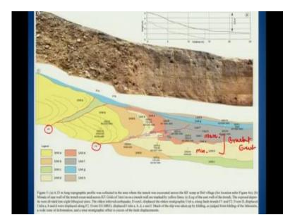
So, this is a photo mosaic of the trench, which was escalated across this curve here and which goes almost like about 10 to 15 meters and this is the topographic profile we have and the trench portion has been marked by the dotted box here and after mosaicking the photographs you can prepare a detailed sketch, but this be we did as I have discussed right in the beginning, that we did the sketching of the trench precisely using the grid in the field on a graph sheet.
