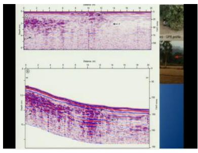
So this was the GPR profile, this is not I would say that this is a raw profile, what we took this not processed at all. But this is not for further, we added the topographic corrections to this, as well as the slight processing part. So after processing, we clearly see the low angle fault cutting and the deposits young deposits and since we until we are unable to open we will not be able to say that this is young deposits.
