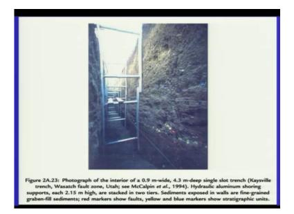
And this is another photograph of that. So you do lot of detailed mapping and before getting into the mapping, you need to clean all the walls and all that and by brush you can do that. So usually we use the painting brush and very fine and with the soft hand. We do not apply much pressure, but with the soft hand we keep on cleaning the wall very precisely and also this top surface has to be clean very properly.
