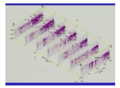
Now with the help of GPR survey, you can also perform three-dimensional mapping and that what we did. The grid has been shown here. So this is the grid which we took almost 20 meter by 6 meter here and we took multiple profiles and when we club this. So the previous one was 2D profile, we have and this is the 3D profile in the area of interest what we wanted to do and this also helped us in identifying and interpreting the depth of the fault with changes.
