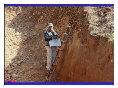
So after that you need to do the detailed mapping, which has been shown here. So in some time, if the walls are little high then you have to use the ladder, which helps you in measuring the units precisely. So this trench if you see is almost like 1/2 meter here 1, 2 and almost 3 meters deep. So as I am emphasizing that we need to do lot of mapping here.
