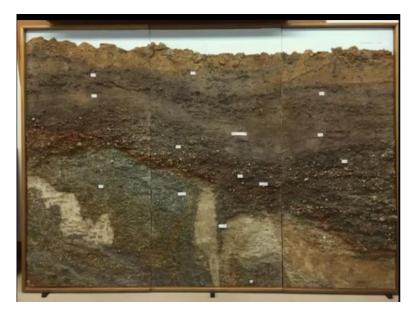
So you can have peel and then you can mosaic it, which can help you in preserving this in lab. This is one of the greatest advantage of this technique that you can bring home or bring back in your lab the whole trench lock. So the fault traces here, it goes up to this one and you can see that deformation and the deposits.
