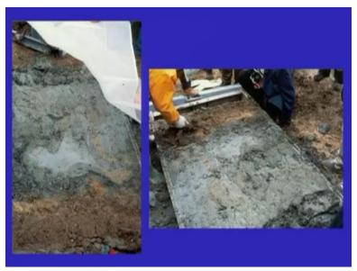
So what we see is that, you will be able to have the complete log of the trench in no time and you can clean it and you can put the net or fine net cloth, cotton cloth and you can have the peel of that trench wall also.
