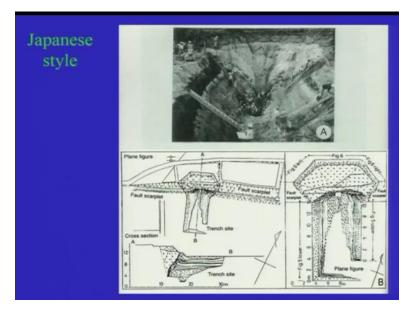
Now another style of the trench as compared to what we have seen the single slot trench of US, the Japanese trenches usually have been seen, they open very wide trenches and one basic parameter which they include is that they keep the walls inclined and this is for the safety purpose and with the inclined trenches you can go deeper and the sketch of the plane view of the trench which has been shown here.
