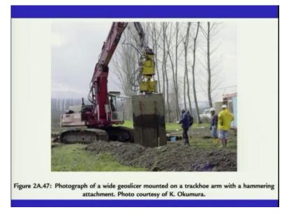
This is being done in Japan, mainly what we call the geoslicer, but sometimes this is not so good in the sense because you may not be having the good site to put the geoslice, if you are having very coarse deposits. So what has been done that you have in a very thick metal sheet here, which has been pushed down into the surface with the help of crane and the vibrator, which has been mounted here and this of course is an expensive affair.
