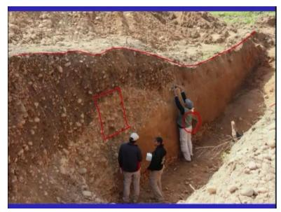
Then, as I told that you have to do after the cleaning, you need to do lot of measurements and you need to have a proper grading, which has been shown here and that is what we are doing is, we are measuring the attitude of the fault. How much the inclination has been seen that is the depth of the fault and what is the amount of displacement, when you fix up the different units. So this is the wall, how you should put it very clean.
