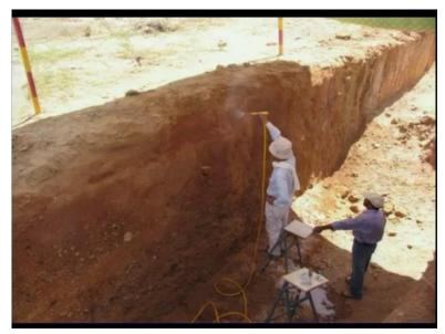
And as I told that in Japan, mostly what we do is, we put lot of water on the wall and but sometimes this is not very good in the sense, because that that may result in to the collapse of the walls okay, but this spraying putting water here will remove the finer sediments, which are getting coating or which are coating the different layers and that may result into misinterpretation or while demarcating the different units.
