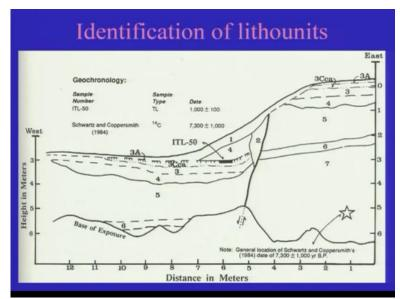
Identification of lithounits will play an extremely important role, because that will help us in identifying different environment as well as the amount of displacement, which we will be able to measure between different layers.
