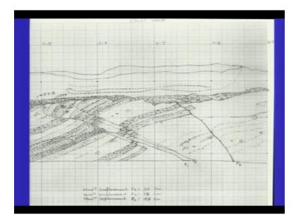
So you can have a very beautiful sketch, which you can prepare with the help of the detailed measurements, you do and this can also help in understanding the pattern of deformation along different fault trench.
