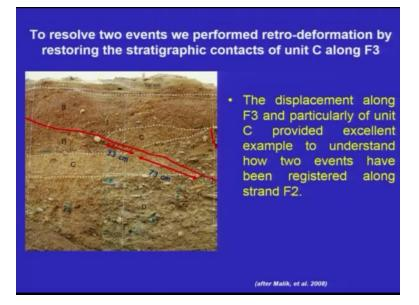
So trench at Lodai, this was the portion which we took for our further interpretation and what it shows here again. So you have the same log here, which we have cut and we tried to retro deform. So we perform the retro deformation by restoring these stratigraphic contacts of C along F3 fault. This was which is marked here is your F3 fault. So along this, what displacement we saw that as I have explained that it was 33 and 73, then how what exactly this tells us.
