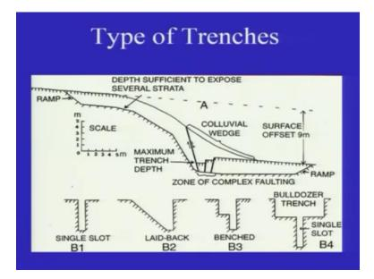
And type of trenches in different areas, if you look at then you can have the single slot trench, then laid-back trench, you have the benches which we have discussed and then you have the bulldoze trenches within single slot which goes for the deeper part. So the ideal way is to open the trench is your across this scarp that is transposed to this scarp and the portion where you exposed the fault, you can go deeper in this area.
