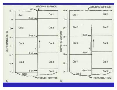
Then coming to the another part that we usually see that in multiple events, you may see that in the top portion the ground or in the up tip part of the fault, you will have minimum displacement. When you go deeper, you will able to see the displacement increases and the another one which is important is that the event horizon. So the last earthquake if you consider that this was the fault and this has displaced the Qal to unit, but has not displaced the qal1.
