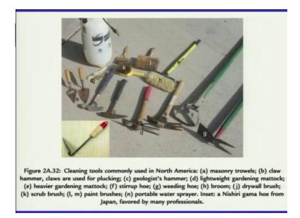
So these are the different tools, which you should have with you, like you have the hammer which is common, then trowels you have, you should have brushes to clean and then to some extent you can even use the water to spray on the wall that will help you in differentiating between the different layers. If you are, suppose you are having the clay layers and the self layer or sand layer, then the absorption of water by different layers will vary.
