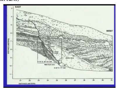
So this trench again, it shows in the normal faulting environment, which shows the angular gravels and then you have the stratified material here and which has been marked in this sheer
