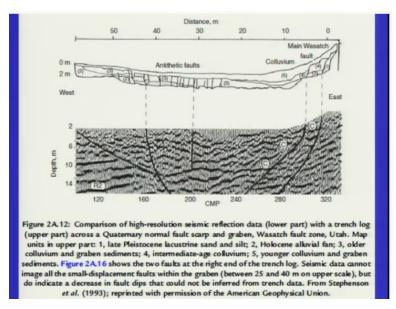
Then you can also do the high-resolution seismic reflection when compared with the trench lock. So this has this trench is hardly 2 meters but with the seismic reflection you are able to reach right up to 14 meters or so on.
