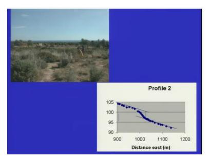
Further now we have started using the total station which keeps the millimeter accuracy points and this will give you this points what we will get will be having x, y and z. So you will have the coordinates of each point which will be given here and with the help of the best-fit line which has been drawn here you can talk about the height of the scarp here.
