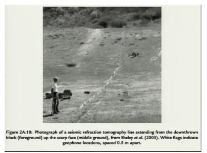
This is an example photographs which has been seen for the seismic reflection tomography where the; you have the tomography line extending from down thrown block in the foreground and the up face scrap in the middle here which goes right up to the top. So this is the scarp here this portion is up this is down, and this is what has been done for the seismic reflection.
