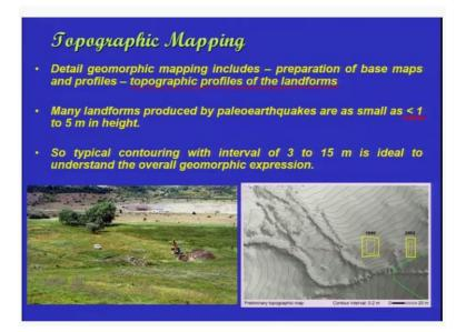
So the most essential which comes with the base maps and all that is your topographic mapping in the field. So detailed geomorphic mapping includes preparation of the base maps and profiles and mainly we are talking about the topographic profiles of the landforms that means your deformed landforms.
