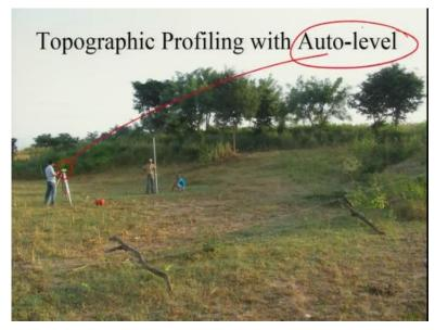
So earlier we used to have we used to do the topographic mapping using auto level. But now we have with the more development in science and technology we have high resolution total stations with which we can generate a millimeter accuracy and maps.
