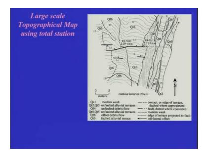
So topographic mapping in the field is extremely important and there is another map which shows from us with the contour interval of 20 centimeter which helped in identifying the displacement of the terraces.
