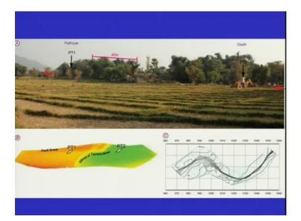
Then after this we go for trenching but this is an one more example where we wanted to map the displacement along this curve or along the surface or sorry displacement of the surface along the fault and the offset of this stream along the fault okay and this what we did we took a number of points with the help of total station and with the simple triangulation we have generated this offset of stream.
