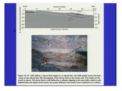
So this is an example of the ground penetrating radar profile which has been shown here they have they have been able to go up to 15 meters so much better than what was been done in seismic reflection and further was it was been compared with the trench which was been dug in this region so this is the logged area which has been seen here and which shows that clear-cut displacement here.
