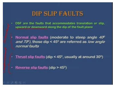
So normal faults that usually has been seen but if you are having steep angle moderate to steep angle usually which ranges from 40 to 70 degrees and those dip with less than 45 degrees are referred as low angle normal faults. Thrust faults if the tip of the fault plane is less than 45 degrees so if you are having for example you have the reverse fault. So this block has moved up so if this angle of the fault is less than 45 degrees then they are termed as thrust faults.
