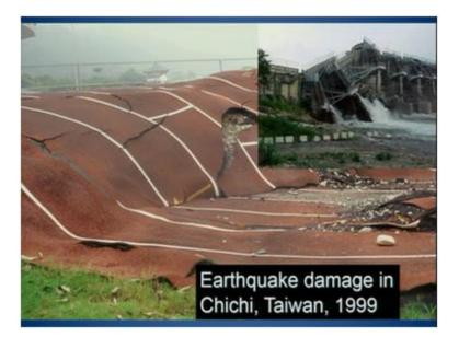
Then this was 1999 chichi earthquake in Taiwan which shows the fault scrap here, so the this was the deformation was manifest rated or the manifestation was seen and passing through one of the the pavilion and the running track which got displace, and default again then the damage here again of the garage.
