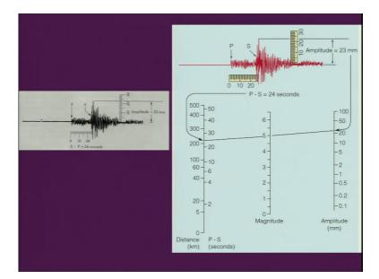
So, basically if you are having the seismograms. So, the difference between the arrival of P wave and S wave has been taken into concentration and that helps and along with that the amplitude has been taken into consideration. So, the example which has been given here, where it shows that you have considered the amplitude of the arrival of the different seismic wave, but mostly it has been taken as an S wave arrival, because this will return to the major deformation.
