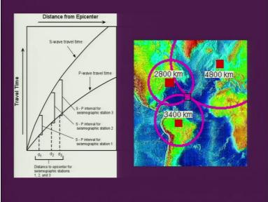
So, if you this are standard diagram, the curves which are available, which helps in locating the earthquake. So, you have the, if at least you have the arrival time difference between the arrival times of P and S with 3 different location you can calculate the distance and that distance is you are would call the radius can plot it based on that and that the intersection of this 3 points will 3 circles will give you the epicenter.
