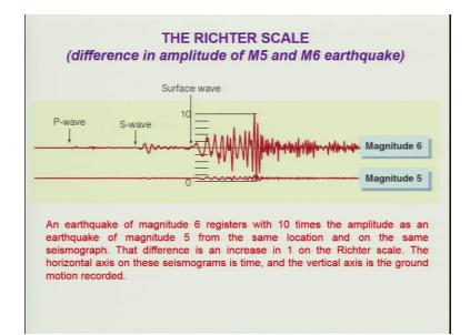
So, the Richter scale if you take the because the amplitude will play an important role what we are seeing here the difference between the magnitude 5 and 6 is very large and that what is spin and we all know that the magnitude if we have between 5 and 6 then the energy which has been going to be released will be almost like an factor of 30. So, here we have the magnitude 6 amplitude, which we see here is quite comparatively larger as compared to what you have the magnitude 5.
