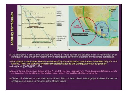
So, locating earthquakes basically you have like 3 locations which are one given here. So, you have 1 station which is sitting and SOCO then TEIG and SSPA. So, these are the 3 stations which were used to locate the epicenter of 1 particular earthquake here. So, what it shows on this curve here or this graph that you are having the distance here this is you are the time difference. So, you have the first P wave which is arriving here was at 1.5 minutes.
