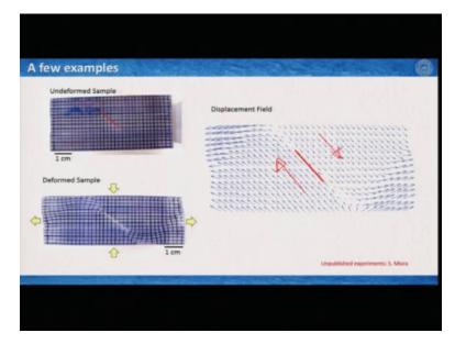
So here is an example of experiments that I performed in the laboratory. What do you see in this undeformed sample? This is a polymer (PMMA) polymethyl methacrylate, it has a cut in the middle like this and then I made some grids, square grids, each grid is about 2 millimeter squares, and then I compressed it. And when I compressed because of this cut in the middle there are some distortions in the deformed sample.
