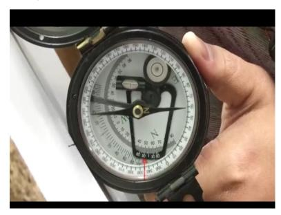
When the bubble in the elongated level have come in the centre, the dip value is the value with which the 0 mark in the vernier coincides with the 180-degree graduated scale and in our case the dip is 55 degrees.
