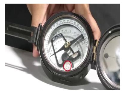
The horizontality of the compass is ensured when we know that the bubble in the circular level is in the centre which is now the case. In order to note the reading, it has to be carefully kept in mind that the, we would take the reading of the northern end of the magnetic needle to which it is pointing in the 360-degree graduated scale. When the pointed arm is pointing towards the direction towards which our thumb was pointing.
