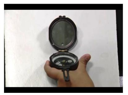
So now put this edge to measure the dip direction against this plane and in the strike line. So the edge is placed against the strike line and now we measure the dip direction. As we know from right hand rule the dip direction would be 220 plus 90 so 310 degrees. But we still would confirm it. So, in order to confirm it, the compass position is this and now we will make it horizontal.
