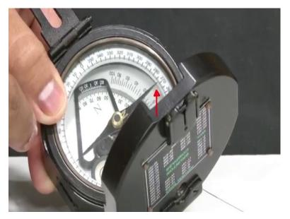
Once we achieve this position, we take the reading which is the value with which the northern end of the magnetic needle points in the 360-degree graduated scale. In our case the value comes out to be around 270 degrees.
