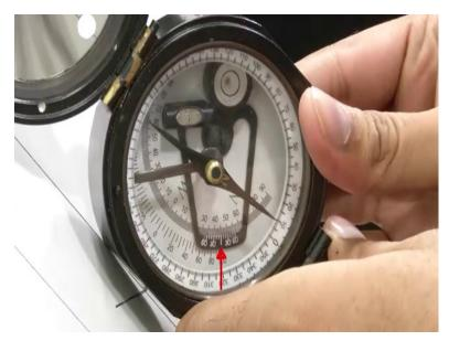
When the bubble in the elongated level will come in the centre we will note the value of plunge in the 180-degree graduated scale to which the zero mark of the vernier will coincide and in our case the amount of plunge is 44 degree. So, thank you all for watching this video and please stay tuned for further videos.
