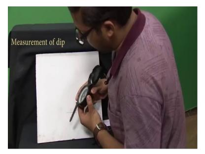
Now, we place the compass perpendicular to the previous position so that this plane is perpendicular to this line. When we ensure this plane is perpendicular to this line this position is sure, the pointed arm will point towards the down dip direction of this bed. Then we will adjust the back lever of the compass so that the bubble in the elongated level comes in the centre.
