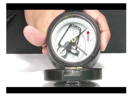
Once we have achieved the horizontal position in the compass, we would take the note of the northern end of the magnetic needle. So, we now see the circular bubble in the circular level is in the centre and our pointed arm is pointing towards the down dip direction and the northern end of the magnetic needle is pointing towards 310 degree in the 360-degree graduated scale. So, the dip direction of this planar feature is 310 degrees.
