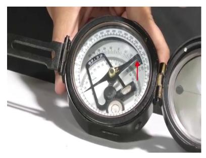
So, when everything is ready bubble is in centre, the northern end of the magnetic needle reads 220 degree when the pointed arm is pointing towards the direction in which the thumb was pointing. So, the strike in this present case is 220 degree.
