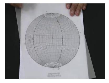
Now, in this problem we will first mark the fracture plane or otherwise the profile plane of the fold. So the profile plane of the fold dips 60 degree towards 280 degree. So, west corresponds to 270 degree so 280 degree is this mark which I have drawn. Now, I make the 280 degree on the east west limb and calculate 60 degree. So, this is 10, 20, 30, 40, 50, 60. So, this grade circle is basically the profile plane of our concern fold. Now, we have marked the profile plane of the concern fold.
