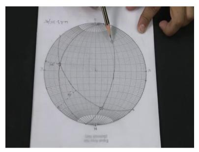
So, now, I rotate the overlay. So we have found the orientation of one of the limbs. Now we count the streak east corresponds to 90 this is 100, 110, 120, 130, 134, 135 but considering right-
