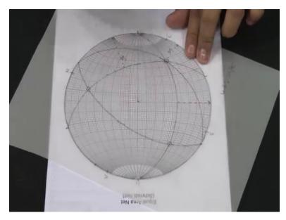
So we will find the grade circle passing through this point by rotating the overlay. Probably we have arrived at the same grade circle. Yeah, so now we will join these two points. So the grade circle that passes through, this is the other strike and we mark the dip. So the dip is 5, 10, 15, 25, 35, 45.
