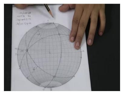
So, now, I again rotate the overlay and read the strike. So the dip amount is 45 and the strike is north so this is 20, 30, 40, 50, 60, 66. So the limb two we have 66 degree is the strike and the dip amount is 45 degree. Clearly, this is the fold axis so the fold axis is plunging 30 degree in direction of 100 degree. So, the orientation of the fold axis is plunging 30 degree and the orientation is 100° and clearly this is our axial plane. So, the axial plane we find out the streak.
