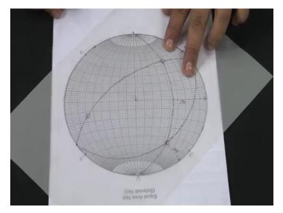
So, now, I rotate the overlay of the tracing paper to find out one of the limbs which pass through the fold axis and also the point we have obtained from the pitch of the limb trace on the fracture plane and clearly, this grade circle represents one of the limbs. This would one of the strikes, and this is one of the strikes and the dip is this, So the dip is 6, 16, 26, 36, 46.
