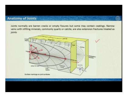
So, here is an illustration that shows what the different features that you expect are in a joint surface. So, joints normally are barren cracks so you will see just a crack surface but with a lot of interesting features. So, or it can be empty fissure but some may contain coatings. Narrow veins with infilling minerals, commonly quartz or calcite, are also extension fractures and you can treat them as joints but let us concentrate on this image.
