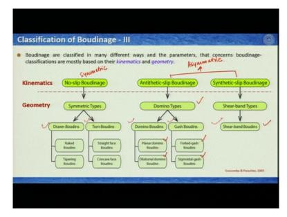
Let's see another classification scheme. So this classification scheme is given by Goscombe & Passchier in 2003 and here they considered both kinematics and geometry. So kinematics means that how do these boudins form with respect to their displacements and so on and we have learned about it. When we were learning the symmetric and asymmetric boudinage. So they define it as no slip boudinage or symmetric boudinage.
