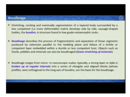
So here are some descriptions that we have just learned. So stretching, necking and eventually segmentation of a layered body surrounded by a less competent or more deformable matrix develop side-by-side, sausage shaped bodies and these are known as boudins. And this is a structure the boudins it generally expects in low-grade metamorphic rocks or boudins generally to form during low-grade metamorphism of the rocks.
