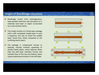
Now how do they form? What is the origin of this boudinage structure? Now people mostly figure out the boudinage structure or most of the structures that we see in nature by experiments. So that also happened with the boudinage. So boudinage mostly results from heterogeneous layer parallel extension and destruction of a relatively hard layer or objects surrounded by a more ductile matrix.
