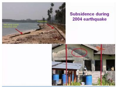
And if you see the subsidence during 2004, so this is an example of that so, the wall along the coastal road before 2004, the area subsided and then they construct the new walls, so this is the present day wall which has been constructed to protect the erosion of coarse, the height of the Tsunami was almost like 3 metres here.
