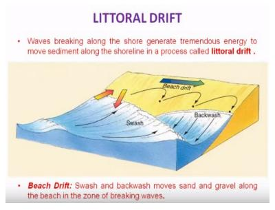
Now coming to this part of the littoral drift usually what we see is the wave waves breaking along the shore generate tremendous energy to move sediments along the shoreline in a process called littoral drift. Now this littoral drift in different location will allow us to see the formation of different landforms. So the red arrow shows the wave action and the back flow or the backwash of the waves which will result into the formation of beach.
