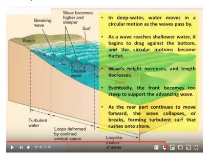
So linear motion so this is what it shows not if you have you are in the deeper part then you have where the motion is almost circular in the deeper waters. As a wave reaches shallow water it begins to drag against the bottom and the circular motion becomes flatter wave height increases and the length decreases. So the wavelength decreases whereas the height of the waves increases eventually the front become too steep to support the advancing wave.
