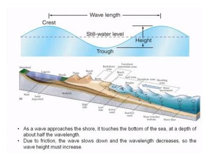
So if you take an complete section of the wave then we have the crust and trough. So most of the waves you will find is with the crust and trough and the important part is that the motion of the waves will vary from the from it location with respect to the coast and also with respect to the depth. So as wave approaches the shore it touches the bottom of the sea at a depth about half the wavelength.
