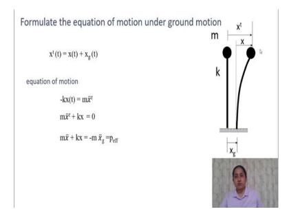
Now, let us look into another system and write the equation of motion. The next system has a lumped mass m and a stiffener k this does not have any damping and the system is affected by a ground displacement Xg. The displacement of this mass relative to the support is indicated as X and the total displacement of this mass has indicated as X t.
