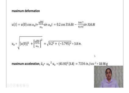
Next we will calculate the deformation of this system. So, you have know the initial conditions, we know the natural frequency. So, you can calculate the displacement as a cos omega n t plus b sin omega t all these values are known. So, you can substitute and get the expression for the displacement of the instrument and you can calculate the
