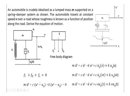
Let us do one more example. In this example an automobile is crudely idealized as a lumped mass m supported by a spring and a damper, and this automobile travels at a constant speed v over a road which has some roughness. So, the roughness of this road can be expressed as a function of X and X is the position of this vehicle on the road.
