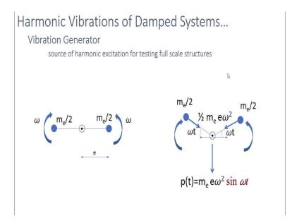
To understand the dynamic properties of structures we often test full scale structures using some harmonic excitation. So, to do that, we need to generate harmonic forces and now we will explore the working of a basic vibration generator.
