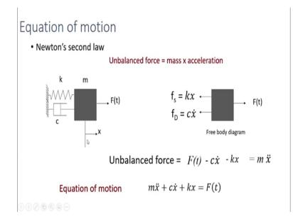
So, first we will make use of Newton's second law to find equation of motion of a system. So, the Newton's second law says the unbalanced force on a body is equal to the mass of the body multiplied by the acceleration it gains. So, this is our single degree of freedom system. So, now, let us isolate this body which is the mass and let us draw the free body diagram of the mass. So, if the system is getting vibrated in this direction because we have a dynamic force in this x-direction.
