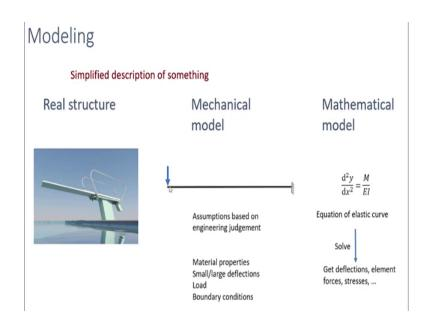
So, what is modeling in the context of structural analysis? So, it means a simplified description of something. So, for example, if we have a real structure, a real life problem so, this is diving board. Suppose, we have to understand the behavior of this structure so, I have to do an analysis of this. So, what is the first step in analyzing this type of system?
