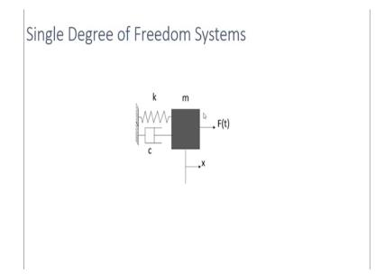
So, the single degree of freedom system can be represented like this – mass can be lumped as a single mass single concentrated mass and there will be a massless spring which is representing the stiffness in the system and the damping. The energy dissipation mechanism can be represented using a viscous damping system with the damping coefficient is equal to c and there will be a force a dynamic time varying force acting on the system.
