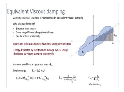
Now, let us use this dynamic hysteresis loop to calculate the equivalent viscous damping in a system. So, in the beginning we discussed that the damping in an actual structure is due to many different energy dissipation mechanisms. And, these mechanisms can be represented by an equivalent viscous damping.
