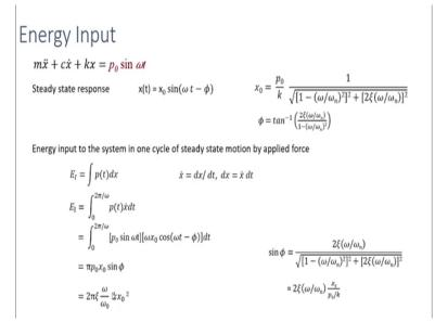
Now, let us see the energy input to a single degree of freedom system under harmonic force. This is the equation of motion of a single degree of freedom system; we have mass damping and stiffness. So, this is the spring force, this is the damping force, this is the inertia force and the sum is equal to the harmonic force acting on the system.
