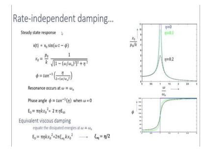
So, let us find out the steady state response. So, this is the expression for steady state response, we need to find the amplitude and the phase angle. So, the amplitude and the phase angle can be calculated again by replacing the value of zeta in the expression for viscous damping response. So, this is the amplitude of the steady state and it can be obtained like p 0 by k. So, this is the static response due to a constant force p naught.
