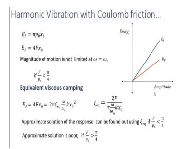
So, we have seen that the input energy to the single degree of freedom system, due to this harmonic force is equal to pi p naught x naught, when omega is equal to omega n that is when the forcing frequency is equal to natural frequency. And, x naught is the steady state amplitude and we also saw that the energy dissipated by friction is equal to 4 F times x naught.
