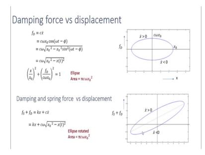
Now, let us understand, how the damping force is related to the displacement. So, we know that the damping force is equal to c x dot that is damping coefficient times velocity. So, we can substitute the steady state velocity and this cos function can be written in terms of sin function. So, we can write this like this. So, this is the displacement at any time t. So, that is x t square.
