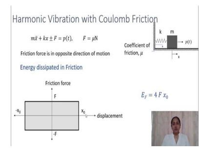
Now, let us see another example of non-viscous damping. So, this is called as coulomb friction damping and it is due to the friction between two surfaces. So, when this mass moves over the surface because of the friction there will be some energy dissipation, we have seen this type of damping during the free vibration case. So, in the case of harmonic vibration the equation of motion as this, m x double dot plus k x plus or minus F is equal to p t the harmonic force.
