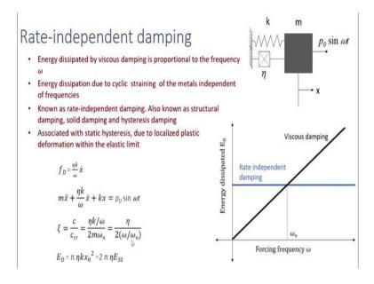
Now, let us see some examples of non-viscous damping. So, the first one we are considering is rate independent damping. So, we have learnt that energy dissipated by a viscous damper is proportional to the forcing frequency omega, but some experiments on metallic structures showed that, the energy dissipation due to cyclic straining of a metal is independent of the forcing frequencies.
