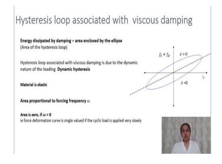
Now, let us look at some properties of this hysteresis loop associated with viscous damping. So, this is the loop we just saw energy dissipated by the damping force that is the viscous damping is equal to the area inside this ellipse or the area inside this hysteresis loop. And, the hysteresis loop associated with viscous damping is due to the dynamic nature of the loading and this is called dynamic hysteresis.
