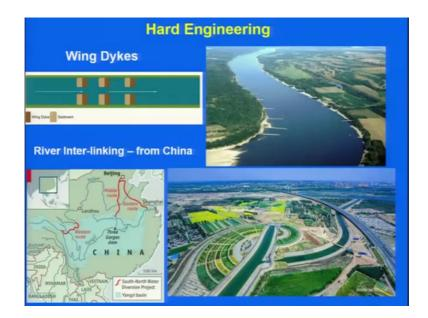
So, hard engineering that is these are what is the wing dykes which have been constructed and there is an example from the on the Chinese river where they have constructed the wing dykes and this also tries to distract the flow ok.
