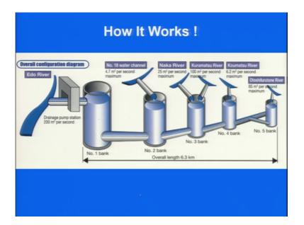
So, this is what how it works actually. So, you have the collection from different channels here the water is getting in. So, these are the names of the different channels which are the tributaries of this main channel Edo channel. And of course, it will be released in the same channel. So, you are not wasting the water, but you are siphoning out the water or in the urban settlements ok.
