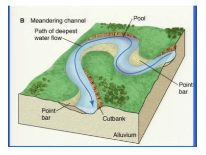
Another one is the meandering pattern as we discussed in the previous one that the outer side will be erosive and the inner side will be depositional side which we call as an point part.
