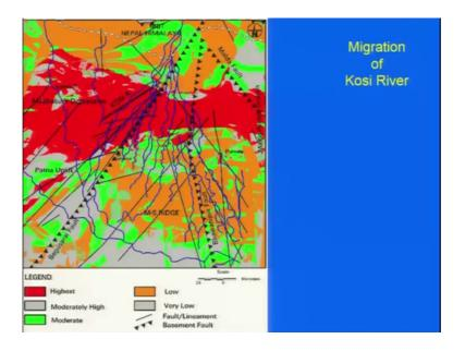
So, you have one is the alluvial fan and this kosi river has experienced or has an tendency of migration from one channel to another one. Some people believe that this fan shape of the kosi is because of the two faults in the region which has resulted into the or played an important role and shaping of the of the fan land from fan like land form.
