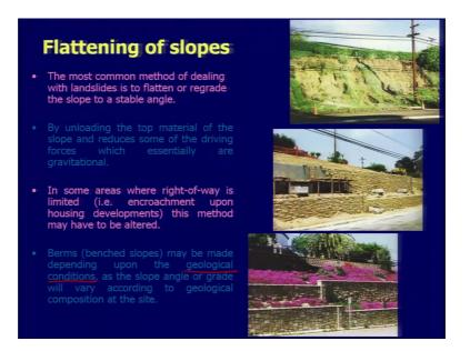
So, flattening of slope very simple the most common method of tailing with landslide is flattening or regrade the slope to a stable angle that, what I have explained in the previous one. That can be done by loading the top material by unloading the top material of this slope and reduce some of the driving forces which essentially our gravitational.
