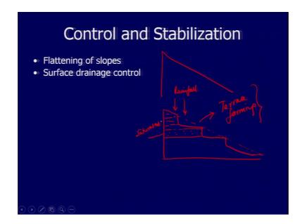
So, control the control and stabilization of slope, the best practice which has been seen in most of the villages is flattening of slope. So, if you go in any hilly areas what you see is basically suppose you are having a slope steep slope here. So, what they do is they will try to reduce the slope.
