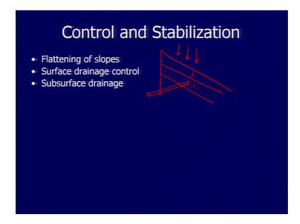
So, if you are having an inclined status, then you have like the succession here. And this is the unit which is short of an what we call vernable unit. And which can slip in future if this becomes saturated. So, the best way is to remove the water as soon as possible through the slope.
