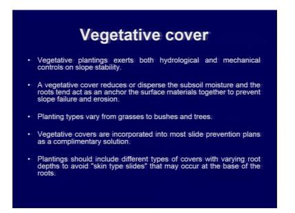
Vegetation cover; now vegetative plantings exerts both hydrological and mechanical controls on this slope stability. Vegetation cover reduces the subsurface moisture and the root tends to act as an anchor. So, this can reduce the chances of land slip increases the stability, but of course, if you are putting very heavy trees on our planting very heavy trees which can put additional load on the slope can also trigger the landslide.
