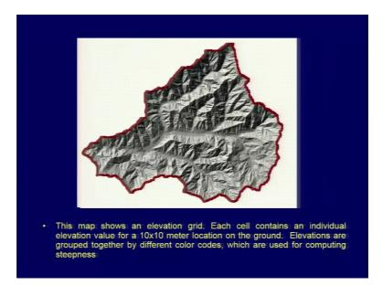
So, this is an in shaded relief map. And you have in GIS you can have understanding with the for the areas and all that you can identify the slopes. And based on those slopes you can also categorize that which area will be prone to landslide.
