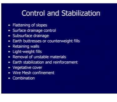
Then you are having the earthen buttress or you can put the counter weight fill. So, this we will discuss quickly then we are having a retaining wall one of the examples we have already discussed. We can have lightweight fills to avoid the slip or to protect the slip or stop the slip further a removal of unstable material.
