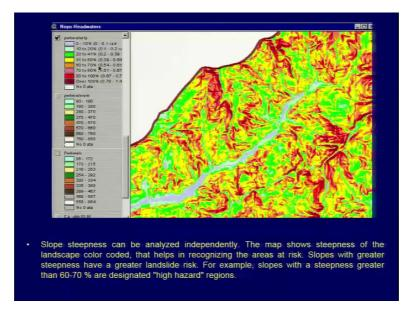
So, these are few maps which shows the classification of the slope. And, you can categorize that which areas will be moderately affected or which areas are under high hazard from the landslide.
