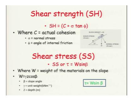
Now, if we take shear strength of the material that can be resolved as C plus sigma tan phi. Tan phi is your internal friction of coefficient and C is your actual cohesion. So, as I was talking that if you are having sand, sand will have this cohesion less.
