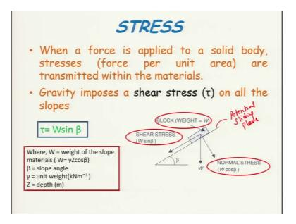
So, stress when a force is applied to a solid body stresses or forces per unit area, because we usually take a stress as an point where the force we are applying per unit area are transmitted within the material and if you take the gravity imposes a shear stress, that is your tau on all the slopes. So, tau is been given as w where w sin beta or you can say its w sin theta, that is an angle of slope and this will be your shear stress.
