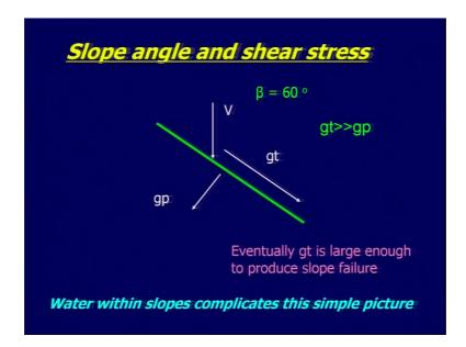
Further if you increase the slope say sixty degrees then you are reducing the gp and you are increasing the. So, you have increased the shear stress, you have reduced the normal stress here. Now in this condition you will have a landslide.
