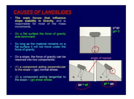
So, causes of landslide the main factor that influenced the slope stability is gravity and is responsible for most of the mass moment. On a flat surface the force of gravity acts downward that is your normal stress. So, if you are having a very flat surface whatever the material you have, you do not have any driving force over here.
