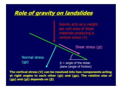
Now, role of gravity on landslides gravity acts as a weight per unit area of slope material producing a vertical stress say V. And we have this as a normal stress and this one is your shear stress and beta is the angle of shear plane along which the material can slip and that is your also will say angle of friction.
