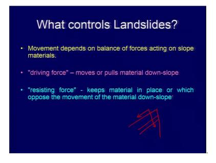
So, what controls landslide? This is the part the moment depends on balance of forces acting on slope. So, as we were talking about that moment will occur under gravity. So, these are the forces which will be acting on slope. So, one is your driving force; which will always tries to move or pull the material down slope.
