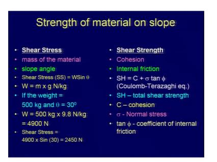
And the shear strength of the material on slope if you take suppose you are having the shear stress, and shear strength then mass of the material need to be taken into consideration slope angle, shear stress, that is your w sin theta vary w is your mass and gravity here Newton per kg now if the weight is say around 500 kg and your theta is around 30 degrees then you have w is equal to your 500 kg into 9.8 Newton per kilogram.
