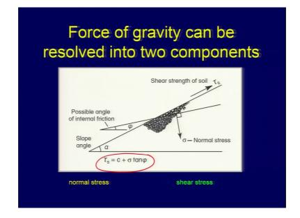
So, force of gravity can be resolved into two components that what we have discussed one is normal stress and shear stress. So, this diagram also explains the same this part will come later when we are talking about the factor of safety where we talk about the coefficient of friction and all that and the normal stress also, and then if you are having and water saturated material then we will have an effective normal stress.
