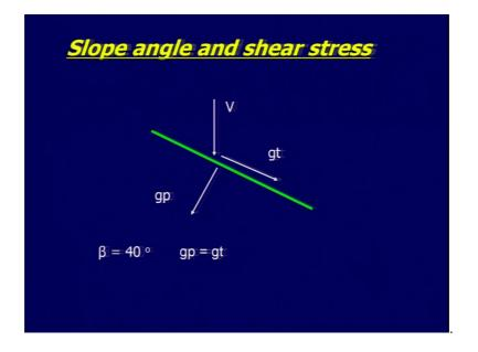
Now, again we increase the slope by about 20 degrees. So, the vertical stress again we are having the two components gp and gt. So, here also we have gp is equal to gt.
