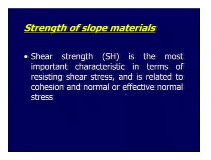
So, if you are having the material; type of material which is porous can hold the water very easily or get saturated that can be dangerous.
