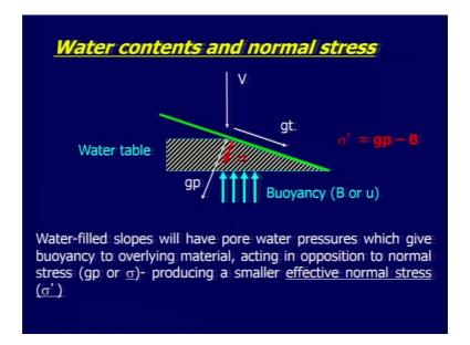
So, water content and normal stress if you take then we have the gp here and if we are having the sigma that is your pore water pressure now the pore water pressure will have some shot o f an buoyancy effect. And that will result into your what has been produced a smaller effective normal stress. So, sigma prime will be your gp what is a normal stress the buoyancy what you are going to do.
