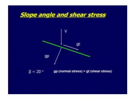
So, suppose you take randomly that beta is equal to 20. So, what is the. So, here the situation is that gp is greater than gt. So, you are resisting force is greater than the driving force here.
