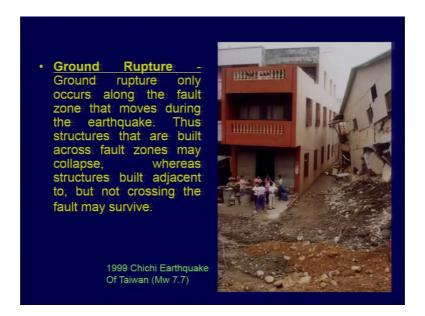
And this is an example of from Taiwan, the rupture pass through this area and this the adjacent house was as it is, but this got damaged because this was been constructed on the default line. So, this is from Taiwan 1999 Chichi earthquake example.
