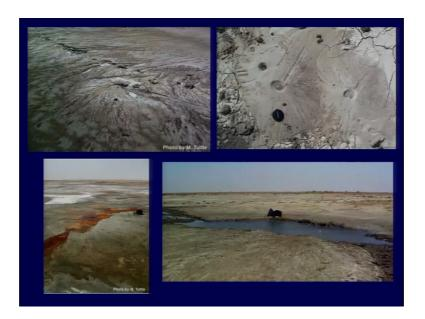
This were these sand blows as I was talking on that day that this typically resembles I have volcanic cone and then along with that we also see a formation of longitudinal fissures and this fissures were also instrumental in pouring out the liquefiable sand, as well as water which was present close to the surface.
