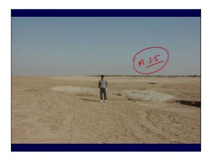
So, what we found was so, this was not only the one sand blow we were having multiple sand blows which we have been observed in this particular region. So, as I told that if you have an ideal condition then you can have the liquefaction even at the magnitude of 5.5, but the shape or the size of the sand blows itself indicate that the magnitude was much higher than 5.5 ok
