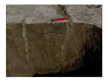
So, close up of that if you see here what we see is this is the contact between the laminated sequence here, pure sand coming here and then in between this within the compute we have some broken fragment.
