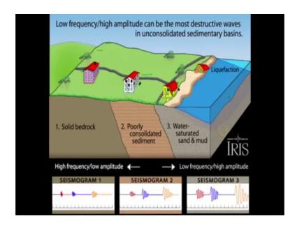
Three consecutive seismograms will show the changing frequency, and amplitude resulting from the change in rock type. The initial P wave arrives with a compressive pump, and rarely causes much damage. Slower shearing S wave introduces a side to side
