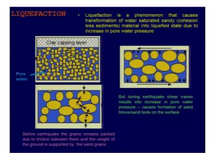
So, for liquefaction what we see here is that we have and uncapping unit, which is not water saturated, which is not porous. As compared to what we are having the porous deposits here, we have a sand. And we are having an very typical bonding nature of the of the sand, and that is an arrangement of the sand grains, and in between the available pores are filled up with water.
