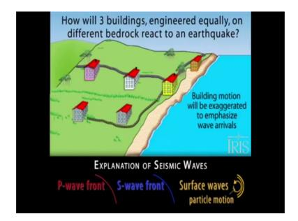
The motion of similar buildings on different bedrock will be exaggerated to show the arrival and compressive P shearing crust, and rolling surface waves from regional earthquake.
