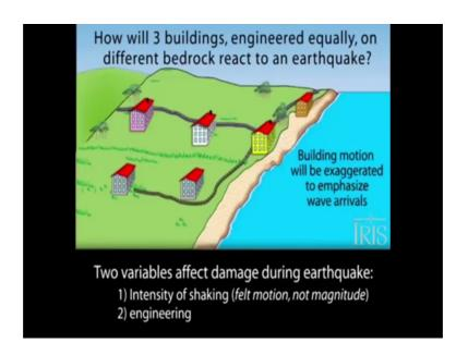
So, this is one short movie which talks about that how will three buildings, engineered equally on different bedrock the react to an earthquake. So, same building with same code, but constructed in three different areas. So, different bedrock how they reacted. So, building motion will be exaggerated to emphasize the wave here it is they have emphasized here, and let us see how what they put it shows ok.
