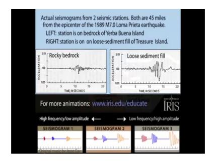
The first seismogram from the pink building on solid ground shows low amplitude, high frequency waves. When the waves hit softer ground they slow down, and increase in amplitude, it is this higher slowing roll that is so destructive during an earthquake.
