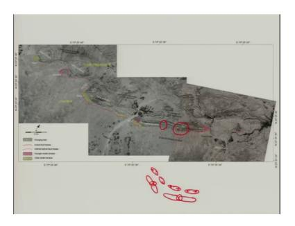
And as I was talking about on that day that this was one of the best site, which we identified for trenching to see the ancient signature of the ancient earthquakes. So, this is an tip of an plunging anticline, which is moving in this direction. So, whenever there is in rupture or displacement on this particular fault that is in south wagged fault, then what we envisage is that this will grow further towards the east.
