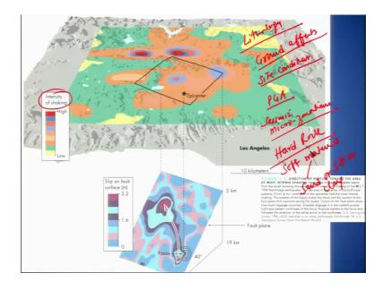
Other than that we go for Seismic Microzonation. So, Seismic Microzonation is extremely important, because not all areas within a region will behave in a similar fashion and that will be in terms of the peak ground acceleration; that is P G A, and this will depend upon the material or the site condition.
