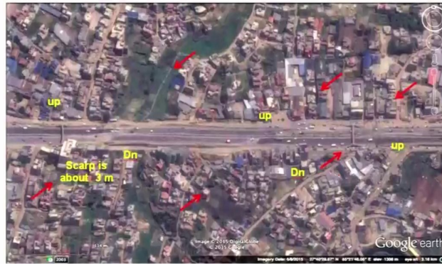
Fig. 7: Google image showing the surface deformation caused by 25 April 2015 Gorkha earthquake (Mw7.8). It resulted into formation of en-echelon fractures developed striking in N60°-70°E. Fractures/extensional cracks are associated with warping of the surface, which has caused relative uplift and subsidence in the deformational zone extending for about 400 m.
