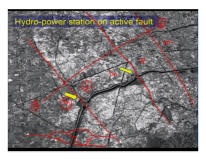
So, these are the two hydro power stations which are been put on exactly on the active fault, the active fault runs here and this is the trace of the active fault and the another traces over here which goes, so you have a very clear boundary because this side is up, this is all I am talking over relative and this side is down and this is down, okay. So, relative to this, this is up actually.
