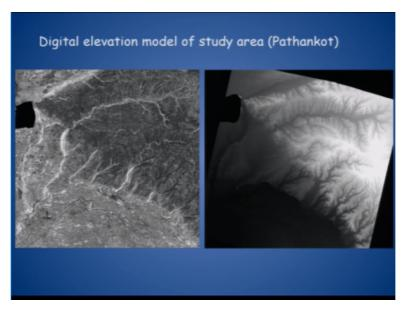
And another representations which you can do is; you can generate the DM from using the after and forward image of the given satellite data and this is the area of Pathankot, now what beautiful things we can extract out of this is that you can easily extract the drainage, okay so even a SRTM data you can use but SRTM data this having better resolution than these SRTM data. So, you can easily the market, the landforms as well as the drainage divides and the drainage network out of this okay.
