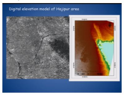
So, this is what I was talking about that you can use the data which is high resolution satellite data to generate different type of illustrations or maps okay, so this again it shows the different elevations and if you clearly look at this part which I was showing in the previous slide which we have marked the lines with COMS are the active faults which; that is the faults which I have displaced the young alluvial plains or flood plain of Beas River.
