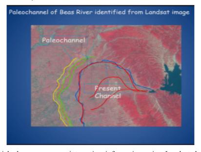
Now, we also picked up some very interesting information using Landsat data, okay so this resolution is around almost like 28 to 29 meters but then also the tonal variations, this image is your fault scrap composite, so you can play with different bands and try to enhance the features okay as per your requirement okay but for us this was the best and which gave us an indication that this a present channel here okay.
