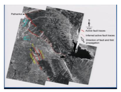
I have discussed this in the previous lectures also, okay now, based on the photo interpretations again we used high resolution satellite data which I have been telling you that we are using CARTOSAT data here but with the stereo vision capabilities ortho-rectified photographs we mark the active fault traces in this region okay. Now, in one of my slide probably, it is next in couple of slides it will come, I am just make a note that this data which we are showing right now is the recent data.
