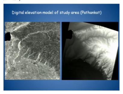
Another we tried with generating the digital elevation model which you can use where you can extract the drainage, this was again using the high resolution satellite data particularly, the CARTOSAT data okay, so this is a raw data and this is what we generated using 2 photographs
