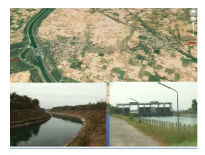
This is the close up of that so, you see in Google Earth, there is a hydro power station, the fault runs here and this is the canal which is cross; which crosses the hydro power station, okay so, whenever there will be an earthquake now, our studies it says that the displacement which is expected on this fault will be almost like 9 meters okay that is the slip on the fault and 3 to 3.5 meter will be a vertical displacement.
