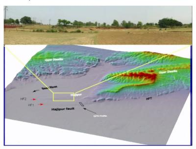
Another one over here, so this is HF2, you can clearly mark that there is an elevation here and a flat area here but this we did not pick up or identify on ground first okay, we used satellite data, we identified this features with an understanding that how the fault scrap will look like and then we visited the field and then we did the trenching and all that okay.
