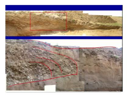
So, these are different topographic profiles which were been collected or obtained or extracted from the shaded relief map, okay. Now, the hazard part here, if you see this curve, if you see or the house sitting exactly on the top of that okay again a mistake, okay further, we opened up a trench and we confirmed that this is an active fault, so these are the signatures of that so, what we see is the fault scrap here and then we see that the formation in the section, okay.
