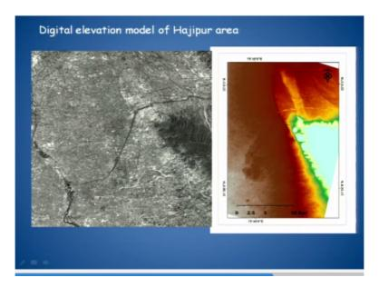
What we found was that 2 hydro power stations are sitting exactly on the top of that okay, at the same time I would like to emphasize here that what we did was; we generated digital elevation model, okay so this is a different form of using the satellite data and trying to pick up your features or the prominent features which exists on the Earth's surface okay. So, what we were talking in the previous slides that a tongue shape feature is this one here.
