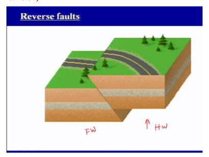
Now coming to the reverse fault. So as we were talking about that in strike slip fault one block will move towards us or away from us along the strike and in combination you will have the movement taking place up along the dip. So here it is reversed what we see in the normal fault. So this is your hanging wall and this is your footwall. So this block has moved up along the fault plane.
