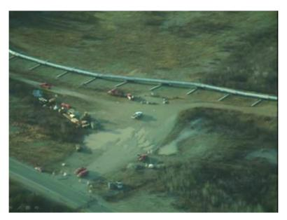
Another very good example from US. Now this fault is named as Denali fault. So what happen was when they were putting and this what you see here a white line is a crude oil pipeline. So they wanted to lay the crude oil pipeline. So all the transit and the orientation the alignment of the pipelines was decided, but they came across that or they came to know that this pipeline will cross the fault line.
