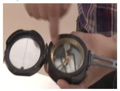
And this is the Brunton compass. In this compass, you have some scales and this compass is used to measure strike and dip on the inclined pins. As you can see here there is a needle which is the needle scripted as n on it so this n is representing the north. So as we move our Brunton compass, this will this needle will also move because this is a magnetic north, magnetic needle. This is following the magnetic north.
