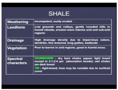
So moving further like what we have the second one is shale okay. Now in terms of the weathering so incompetent, easily eroded okay. In terms of the landforms, low grounds and valleys gently rounded okay, hills in humid climate because of the erosion is more or intense
