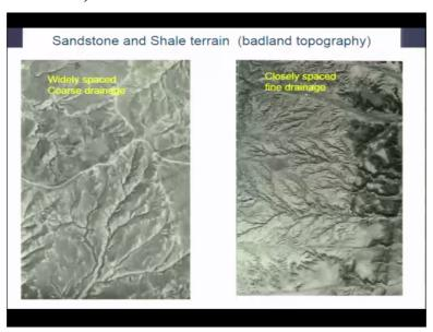
As we discussed, one will be having visible so the sandstone is porous whereas the shale is not so much porous as compared to the sandstone okay. Sandstone will appear brighter; shale will appear darker okay. Sandstone will have widely spaced drainage, shale will have close spaced drainage okay because of it is not allowing the water to penetrate or percolate down and allowing the constant erosion okay.
