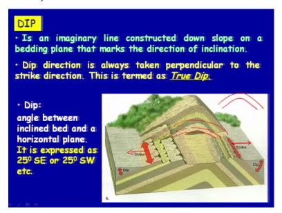
So Dip again is an imaginary line constructed down slope on a bedding plane that marks the direction of inclination, okay. So as I told the direction of inclination; so here you will only be able to give one direction, okay. So Dip direction is always taken perpendicular to the strike direction and this is termed as the True Dip, okay. So if you have the strike direction here, okay say North-South then perpendicular to this will be your Dip direction, okay.
