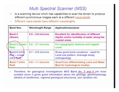
Now, as we were talking about the multispectral scanner or the multispectral data. So, it is a scanning device, which has an capability to scan the terrain to produce different synchronous images each at different wave bands. So, different wave bands have different wavelengths.
