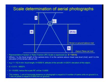
Now, if you take this. But I have slightly simplified it. So, you are having the camera lens here and this is the plane of film and the star the two points which are also on these are on the photograph and these are on the ground here and this is your terrain. So, you are having datum plane at mean sea level for example, you take or any reference plane you take with respect to that you are having the terrain here.
