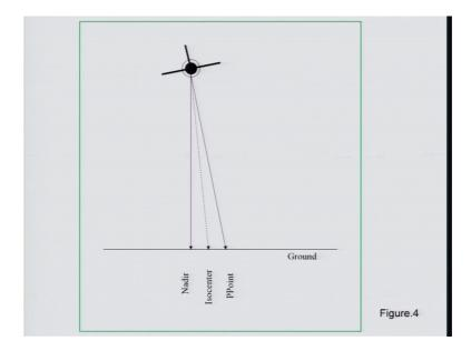
So, this is what we see. So, we have the nadir point will be exactly vertical, but this will be perpendicular to that. So, you have principal point and the nadir point and the center of this two will be termed as isocenter.
