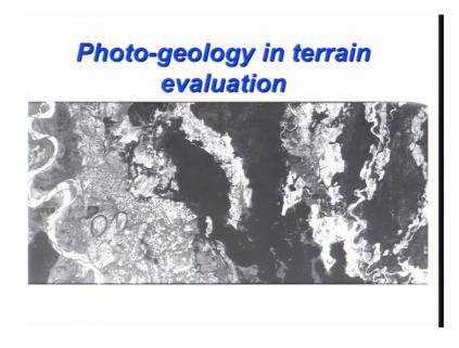
Now, this is and satellite photo, high resolution satellite photo and chromatic data. Corona, this is a Corona satellite photograph of indo Gangetic plain, which shows the darker colors here, could be related to the water bodies and you have the complete range of grey shades which are available here, which can help you and identifying the different features.
