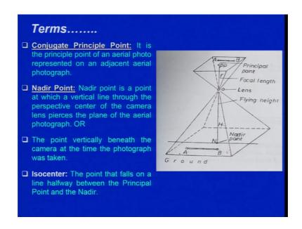
So, terms which we are using conjugate principle point we have already discussed, but we come down to the nadir point. So, nadir point is a point at which a vertical line through the prospective center of the camera lens pierces the plane of the aerial photograph or you can say the point vertically beneath the camera at the time of the photograph taken. So, you have this is the exactly vertical on the prospective center of the camera.
