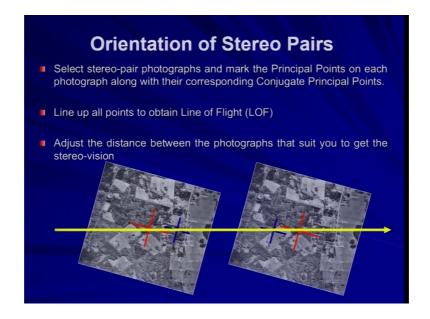
And connecting both that is the stereo pairs photographs and marks of the principle point on each photograph, along with their corresponding conjugate points, line up all points to obtain a line of flight. So, if you connect all this this will be the exactly the line of flight in which you have taken the photographs again.
