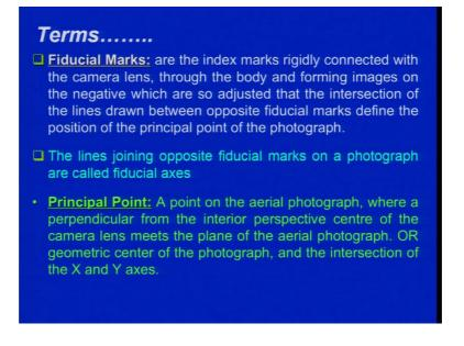
So, fiducial marks are the index marks rigidly connected with the camera lens, through the body and forming images on the negative, that is a framewhich we are having which will create an image on the negative which are so, adjusted that the interacts intersection of the lines drawn between opposite fiducial marks, defines the position of the principal point principal point of the photograph.
