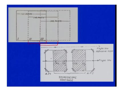
So, this is the if you have a multiple photograph collected and the same direction in a line of flight, then you have the overlap here what has been shown between photograph 1, and photograph 2, and photograph 3, it is almost you can have the overlap here of 60 percent between this, and then you have an overlap of 60 percent between photograph 2 and 3.
