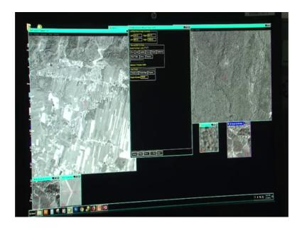
So, now, you know that these are the corrected points and why how to check whether these are the most of the points are corrected or not you can see your maximum y parallax here. So, it has converted into 0.9 to 03 this is little bit accepted to us because it is lying between 0 and 1. It is very difficult to reach to take this factor near to 0, but yes you can do it by taking your time and correcting these points up to the extent what you can do ok.
