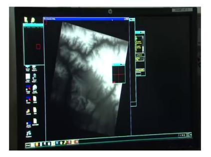
You can see the DEM for those two images has been created and shown like this ok. So, you can see here that these streams are joining the main river channel. So, this is the main river also called trunk stream in form of river fluvial geomorphology this is trunk stream this you must have learned in your geomorphology lectures ok.
