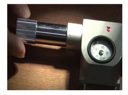
So, this will give you the reading. This is, this and this rod, this bar can be slided. They there are 2 graticules of glass; number 1 and number 2. One is on the left side another on the right side. So, this graticule is more or less fixed with the on this bar. But this graticule you can move by the slider on this rod. So, this is the main scale given inside from 0 to 40 and this your Vermeer scale having a 0 count of 0.01.
