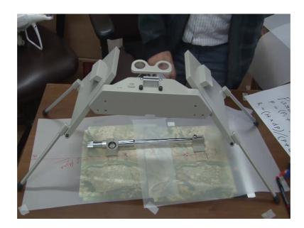
We have already generated 3D vision of this areas under the mirror stereoscopic. So, now, we are again fixing these images in the same manner. So, that they are correctly oriented with the same exercise by coinciding our fingers in this way ok. So, now, this 2 images are in the 3D position.
