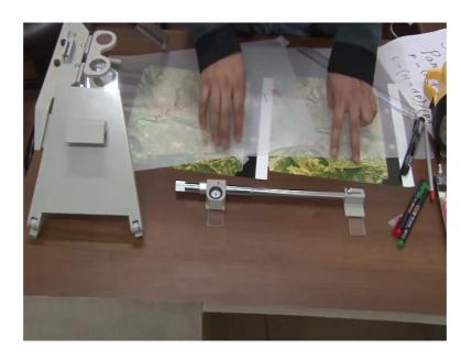
So, this equipment is used with the mirror stereoscope. So, when you place your photograph, the arrear photograph the stereo pair under this mirror stereoscope and then, do the orientation of this photographs fix your photographs. Then, you will put your parallax bar over this photographs to do measurements ok, measurements of the objects or any type of geomorphic landforms. You can take the heights, the measurement of the bottom and top of the those objectives ok.
