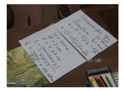
So, please focus on this formula, Stereoscopic Parallax. So, this, in this, this P, P 1 and P 2. This P 1 is actually the distance between the principle point and the conjugate principle point over a photograph and this P 2 is the principle point is the distance between the principle point and conjugate principle point on the second photograph ok.
