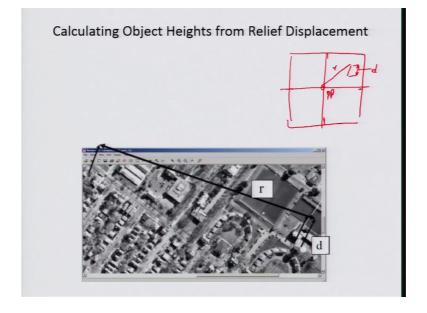
So, again the similar one. So, you have for here it has been given this is the top of the conical building or this structure, and this is the base of that and the distance difference of that is your d and this is your principal point. So, if you remember, we can have the principal points suppose we are having the photograph here and if you are having the fiducial marks on either side you can draw the principal point.
