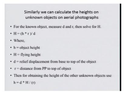
Similarly, you can calculate the height of unknown object on the aerial photographs. So, for the known object measure d and r then small h where, h is the object height as a flying height this you know this is the relief displacement from the base on top of the building r is the radial distance from PP to top of the building or the object then you can have this one obtained.
