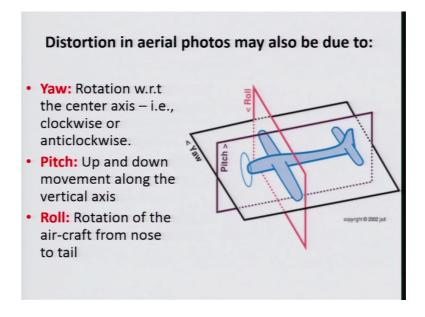
Now, on aerial photographs whatever the data has been collected will show some distortion, and distortion may be due to many reasons, but few reasons which are added on because of the problems, we face in flight either it is because of the rotation, because of the flight moving up and down, and either they are if the flight is moving anti-clock or clockwise direction. So, these are the reasons because of which the scale of the photograph will not be a same throughout.
