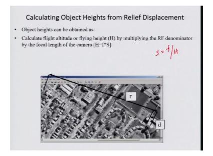
So, object height can be obtained as one calculate flight altitude or flying height by multiplying the this is your ratio fraction by local length of the camera. So, simple we lost in one of the lecture we talked about the scale of the photograph. So, scale of the photograph if you take is S is equal to the focal length of the camera lens by H here. So, with this simple equation, you can calculate the even the height of the flying height and H is your height of the object if you take.
