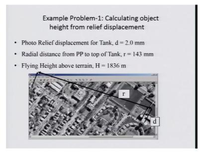
So, another example if you look at the relieve displacement of a tank the similar one for example, you are having 2 millimeter a displacement that is your d radial distance with respect to PP to the top of the tank is 143 millimeter and the flying height is this one. So, you can calculate based on this which will give you the height around 26 meters.
