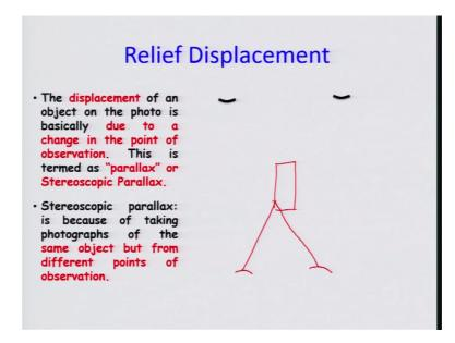
Now, let us look at this example here, the relief displacement the displacement of an object on the photo is basically due to a change in the point of observation, because you
