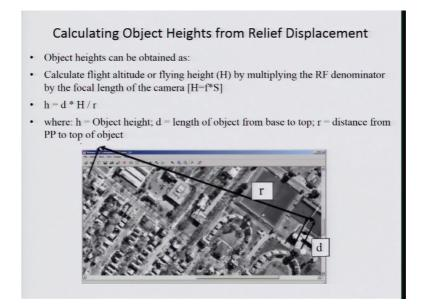
So, you are having d that is the displacement, here that or you can say the displacement of relief from the top of the building and at the base of the building you can take.
