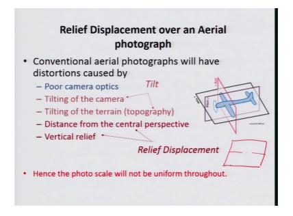
So, these are a few things, which are we cannot help it out while taking the other mission or flying over the terrain. So, relief displacement over an aerial photos conventional aerial photographs, will have distortion caused by poor camera optics, these are add on distortions which can be added, because of the poor camera optics tilting of the camera, now tilting of the camera can also be added because of the rotation of the aircraft.
