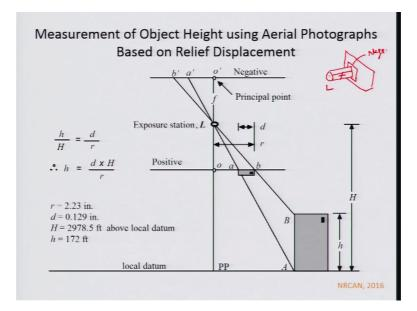
And this is another simplified way, which has been given here. So, d either you call the displacement or the relief displacement, which you will encounter in aerial photographs and can be obtained from the measurement of the top of the object and the bottom of the object.
