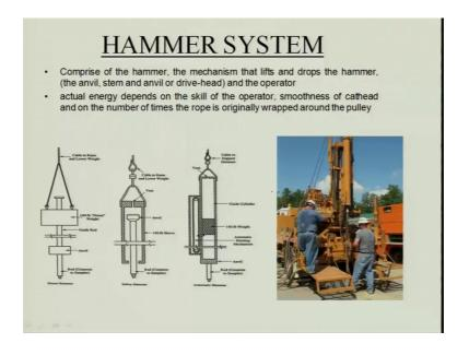
And drop the hammer it consists of anvil system and anvil or drive head. Actually energy depends on the skill of the operator's smoothness.
