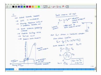
Wall pushed towards back fill. Then what will happen? The soil is compressed, soil is compressed and this shearing resistance built up in the direction towards the wall.
