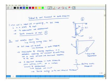
So, let me let me put it particularly when wall is rigid and unyielding, retaining wall is rigid and unyielding, it is neither yielding in translation rotation or any of the mode the soil mass, soil mass is in a state is in a state of rest. In that case soil mass is in the state of the rest what will happen? Particularly this case there is no deformation and displacement. And earth pressure corresponding to this state is called earth pressure at rest.
