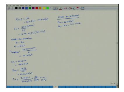
Net ultimate or net safe ultimate C N C by factor of safety because sub soil profile is your purely cohesive soil, there is no 5, it is purely cohesive soil, there is no 5. So, then it comes out to be 145.6 divided by 2.5 whatever is your divide 145.6; I am not putting it a factor of safety q net; I am taking it C N C not safe q ultimate net I am taking C N C which is equal to 26 into 5.6 which is equal to 145.6 Kilo Newton per meter square.
