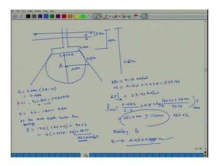
So, it is coming out to be 251.7 mm. So, it is not. So, based on that B value has been modified and the B value comes out to be 4.45, by 4.45 meter taking into this dimensions you can check yourself, this is for you kind of a home assignment; home assignment, you can check whether with this dimensions, whether this foundations is going to satisfy the bearing capacity criteria as well as settlement criteria this is what I have gone through.
