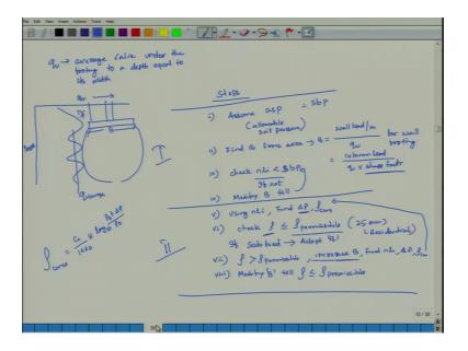
Step one is your assuming allowable soil pressure is equal to soil bearing pressure, find it out, what is the dimensions? Once you get your dimensions then with these dimensions check your permissible consolidation settlement at any stage suppose at any stage if it is not satisfied, then you modified the value of the B. So, this case one example I have solved last class; there is a case and there is a column interior column load is 510 Kilo
