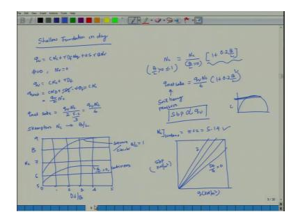
For the case of shallow foundations in clay, I have explained for purely cohesive soils 5 is equal to 0 and N gamma is equal to 0 and it is nothing, but if I write it bearing soil; bearing pressure is directly proportional to your q u there are charts of l label N c verses D f by B and I have also explained there are 2 steps.
