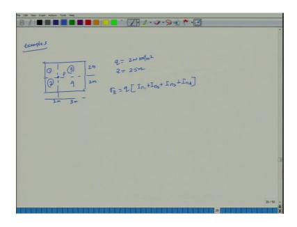
So, I will solve more problems later on. So, example 3 this is your example 3 and this point is your point P inside. So, this distance is point p from here it is your 2 meter here it is 3 meter here it is 2 meter here it is 2 meter, now I if I take it divided in such a way that then this will be 1, 2, 3 and 4.
