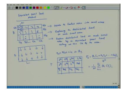
And for square shape or strip footing I have covered then equivalent point method means divide the loaded area into small areas if there is a area B by L into small-small areas.
