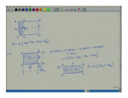
So, first one I have covered go to the second 1; case 2. So, what will happen? So, there is a point somewhere else at point O then in this case it is not equal first principle is I have to divide in such a way that it should be at the corner of your rectangular loaded area; that means, at the corner means if I divide it in such a way that the point O should be common corner.
