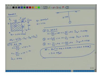
Now, come to example 2 there is a case in this case point p will be located it has been ask to find it out to increase in stress because of your rectangular loaded this at here outside your loaded area at point P. So, as I said I have make it in this arrangement. So, let us name it A B C D then E F P H G.
