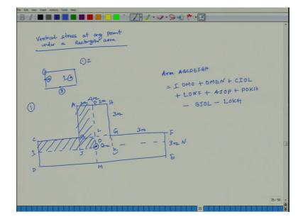
So, based on that I have started one example how to solve it suppose this is the case rectangular loaded area first point load may be anywhere else point of point where your stress you need to find it out. Second, it may be outside the area third it may be one of the phase either B or L it will be there.
