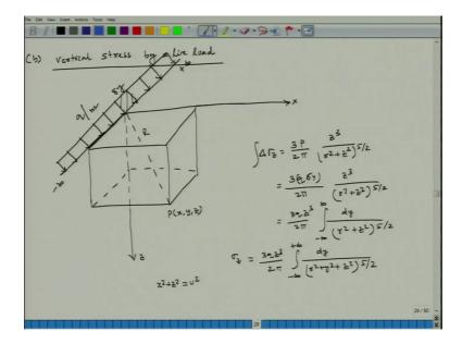
Then considering point load, it has been extended to find it out vertical stress by a line load. Then vertical stress distribution by a strip load again considering point load.
