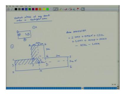
So, like vertical stress, at any point under a rectangular area. It is at any point any point, under a rectangular area means, if this is my rectangular area. Generally, what we have done earlier if this is the rectangular area generally by means of if you go back to here it is at the corner. So, it not necessarily always should be at the corner.
