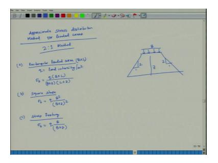
Approximate stress distribution method for loaded areas. These are all point load then there is a strip load, line load, then there is circular load at the center then rectangular load at the corner. Then if you want to find it out suppose there is no chart if we want to find it out approximate distributions approximately what should be the value it is called 2 is to 1 method. It is called 2 is to 1 method.
