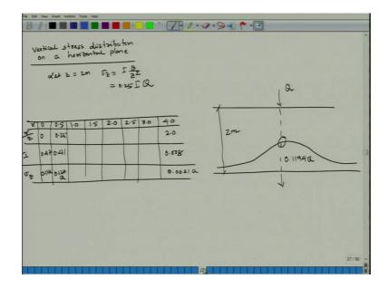
So last class I have covered vertical stress distribution on a horizontal plane. And as well as vertical stress distribution on a vertical plane.
