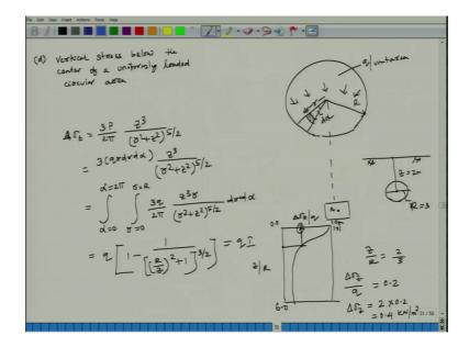
Then is your vertical stress below this center of a uniformly loaded circular area. Again this has been taken into a small strip or small dr and it has been integrated considering as a point load. Then we got a chart, this chart is your delta sigma z by q divide by z by f R, once you know the radius of your circular area and distance below the ground surface where increase in stress has to be calculated then you can calculate what is the increase in stress because of your circular loaded area.
