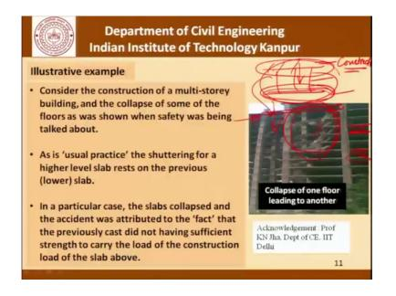
So Now, going back to our discussion on relation of quality and safety we are seen this picture and seen the collapse of these floors while the building was on construction. Now as is usual practice the shuttering for a higher level slab rests on the previous lower slab.
